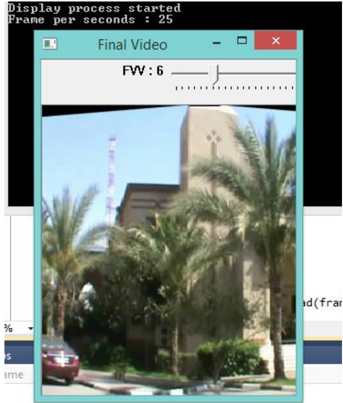
Figure 4-5 FVV system displays stitched video with track-bar for controlling interpolation between viewpoints
