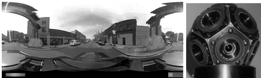
Figure 2-2 Onnidirectional camera and a corresponding spherical view.[5]
